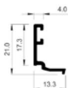
Glazing bead 4mm Triple glazed
